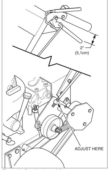
Figure 10. Steering Lever Adjustment
